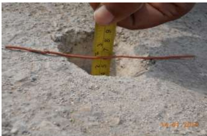
Thickness of asphalt layer checked
